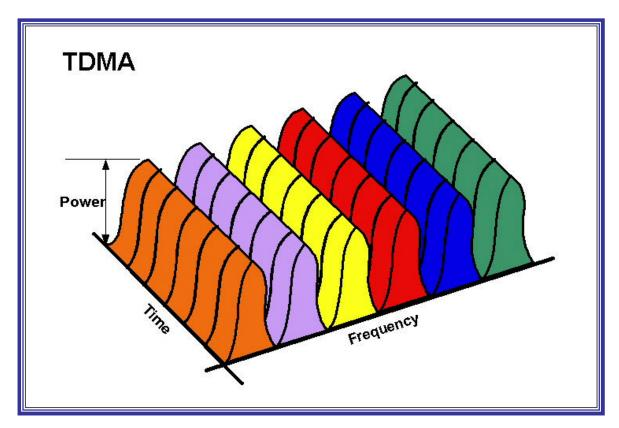
In **Time Division Multiple Access (TDMA)**, it makes use of the same frequency spectrum but allows more users on the same band of frequencies by dividing the time into "slots" and shares the channel between users by assigning them different time slots.
