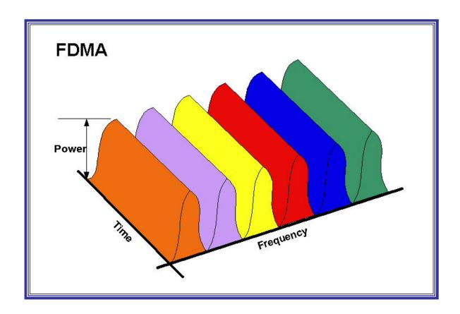
With Frequency Division Multiple Access (FDMA), different signals are assigned frequency channels. A channel is a frequency. FDMA is a basic technology in the analog Advanced Mobile Phone System (AMPS). With FDMA, each channel can be assigned to only one user at a time. FDMA is also used in the Total Access Communication System (TACS).
