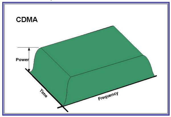
In **Code Division Multiple Access (CDMA)**, each user is assigned a different pseudorandom binary sequence that modulates the carrier, spreading the spectrum of the waveform and giving each user a unique code pattern.
